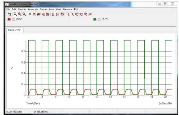
Figure 41. Pulse Circuit Response Displayed in SIMetrix
