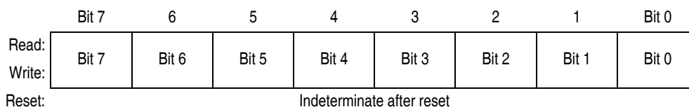
Figure 14-13. TIM Channel Register Low (TCHxL)
