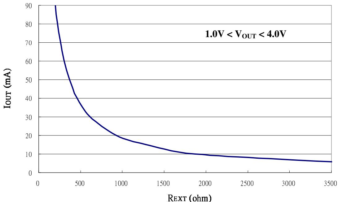
Also, when SCT2210's output voltage is set between 1V and 4V, the output current  $I_{OUT}$  can be set by the formula:  $I_{OUT} = 30(630 / R_{EXT})$  mA. Thus the output currents are all set to 21mA ( $\pm 6\%$ ) by set the reference value  $R_{EXT} = 900\Omega$ .
